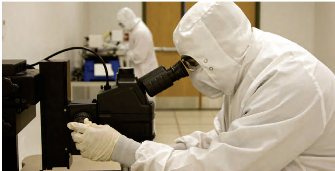
Those who work in the $6.5 million cleanroom must wear protective gear to prevent particles from possibly destroying the miniscule devices that are being created.
